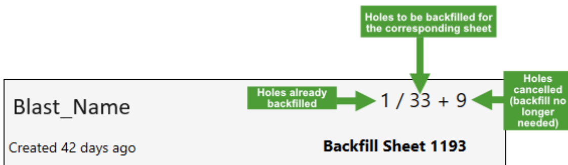
Figure 9-2 The backfilling state of holes in a blast
